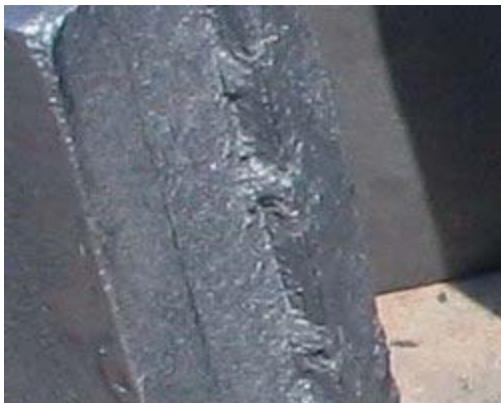
Sand Burning Defect
