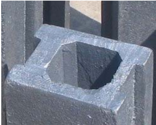
Raised Mold Defect
