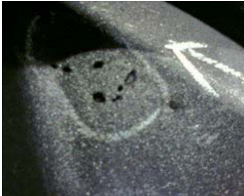
Shrinkage Cavity Defect
