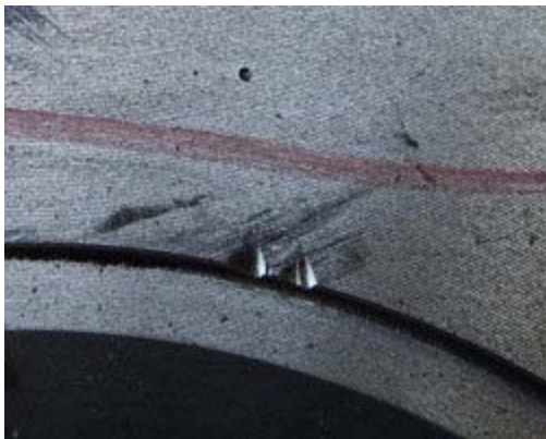
Mechanical Damage Defect
