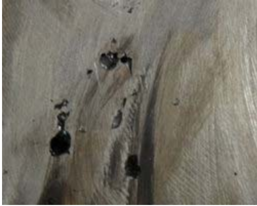
Sand Inclusion Defect
