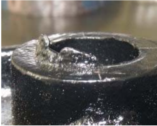
Joint Flash Defect
