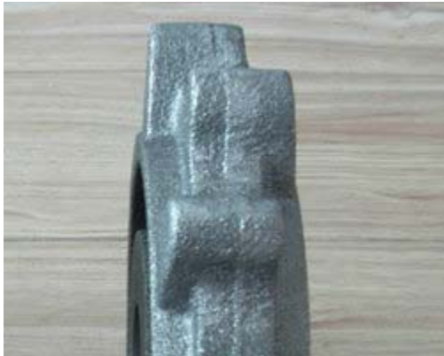
Mismatch Mold Defect
