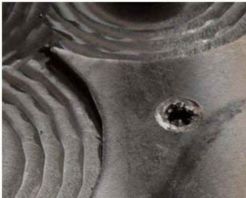
Uneven Hardness Defect
